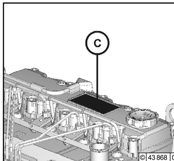
The company plate **C** is fixed to the valve covering hood.
