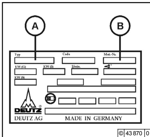
The engine type **A**, engine number **B** and the power data are stamped on the company plate. The engine type and number must be stated when purchasing spare parts.
