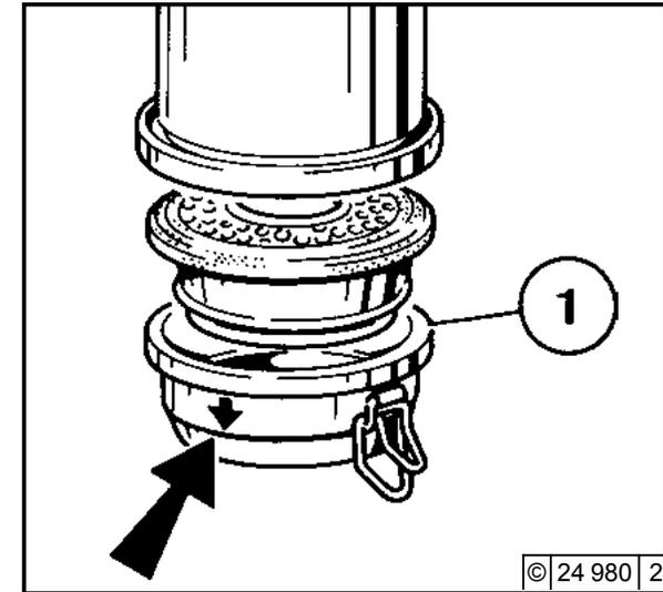
Fill the oil pan 1 of the oil bath air filter with engine oil up to the arrow marking.
