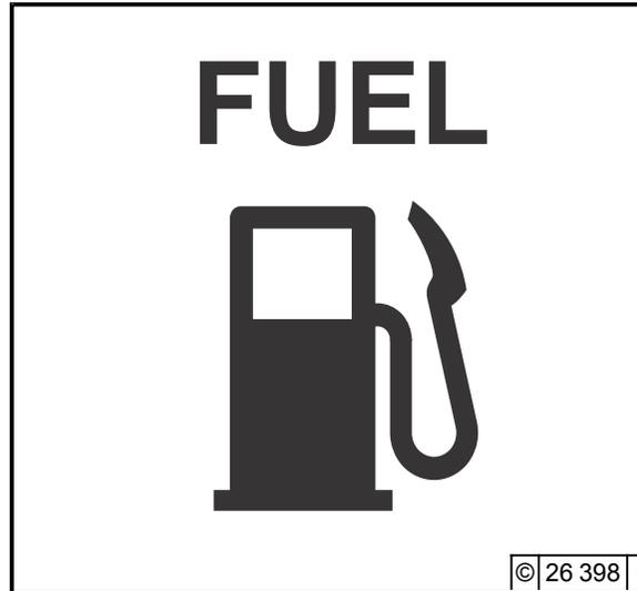
Only use standard branded diesel fuel. For fuel quality see 4.2. Depending on the outside temperature, use either summer or winter diesel fuel.
