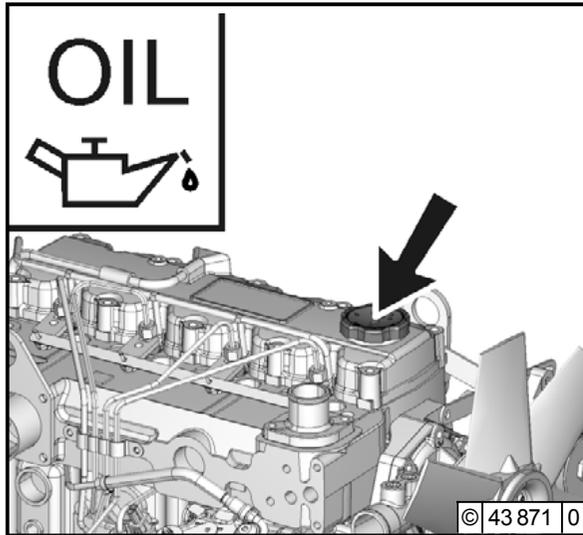
The engines are generally supplied without oil filling.
